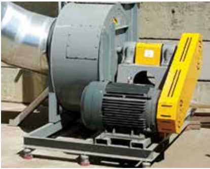
45kW High Efficiency Centrifugal Fan
