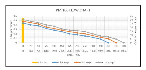
NOTE: There are numerous factors affecting the cycle rate, and therefore' flow rate of air driven liquid pumps. They can be, but are not limited to, air-compressor performance, air-line restrictions and the icing-up of the exhaust.
