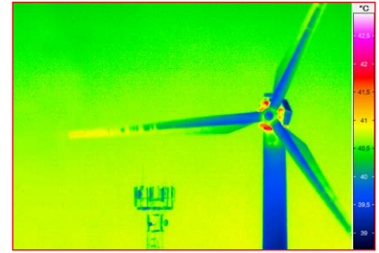
Rotating rotor blade of a wind turbine
