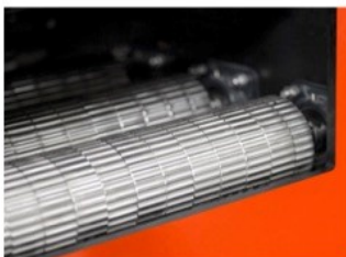
Large diameter driven hold downs.
