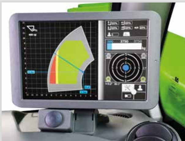
Merlo ASCS (Adaptive Stability Control System) rated capacity limiter
