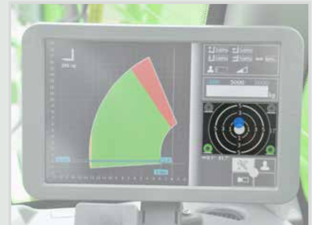
Lateral and longitudinal level indicators
