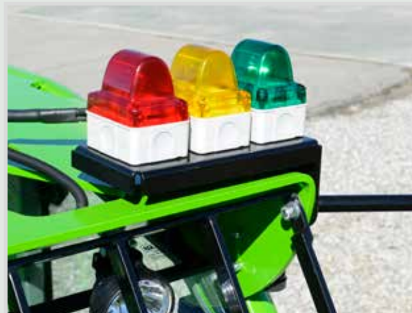
External longitudinal stability indicator
