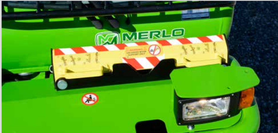
Boom ram safety blocking device
