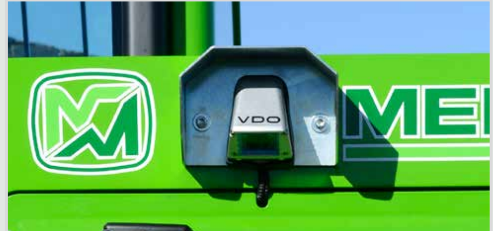
Rear camera starts automatically when engaging the reverse shuttle.
