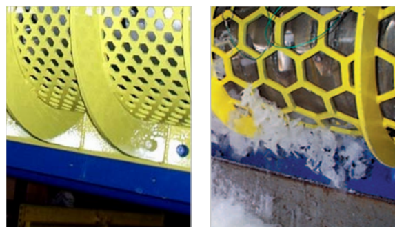
Optional screens available with openings from 1/2-inch to 8 inches (13-203mm)
