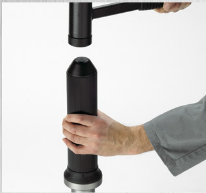
Correct operation of the tool for mounting ball bearings.
