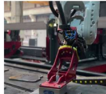
ROBOTIC STRUCTURAL STEEL ASSEMBLY
