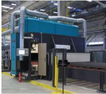
SHOT BLASTING & PAINTING SYSTEMS
