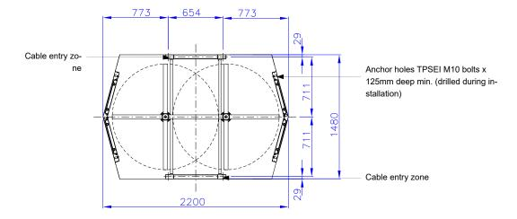
Concrete Base to specification at least fck (cube)  $30N/mm^2$  of resistance Base to be flat and level to +/- 5mm over footprint area. Dimensions to be >  $1800 \times 2400 \times 150$  deep min (units in mm)
