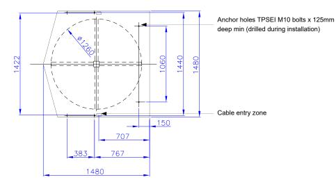
Concrete Base to specification at least fck (cube)  $30N/mm^2$  of resistance Base to be flat and level to +/- 5mm over footprint area. Dimensions to be >  $1800 \times 1800 \times 150$  deep min (units in mm)
