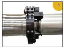
Detach press-tool and move press collar to position 2
