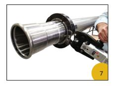
Attach press-tool, check full insertion and press
