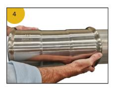
Assemble fitting onto tube to full depth, correlate with witness mark
