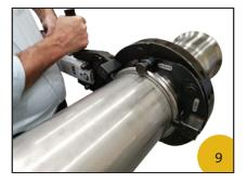
Attach press-tool and press
