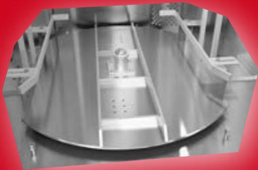
New ball coupling which facilitates coupling between the resting rack and the platform. A magnetic detector ensures correct functioning of the carriage stops. Optional universal platform.
