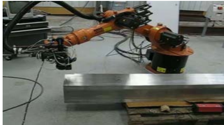
LASER WELDING WITH SPOT-IN-SPOT DESIGN
