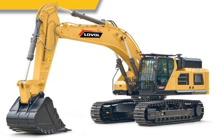
The LOVOL 56 tonne ALFA series excavator features a Deutz Weichai engine with the renowned, reliable and efficient Linde hydraulic system. Pilot oil operated joysticks for precision and control with less electrical items. Climate controlled air conditioning. Lined, sealed and silenced cab with air suspension seat and ergonomic layout for maximum operator comfort.
