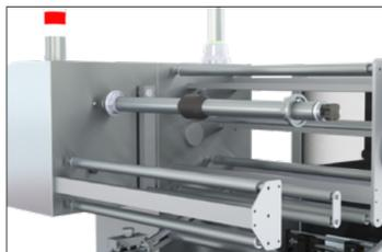
Directly Servo-driven reel shaft (T version)
