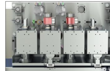
Longitudinal sealing station (B version)
