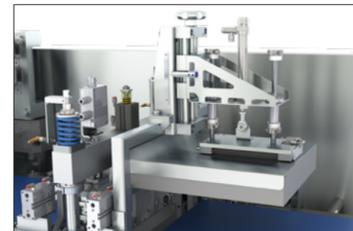
Box Motion transversal jaws with pressure pad
