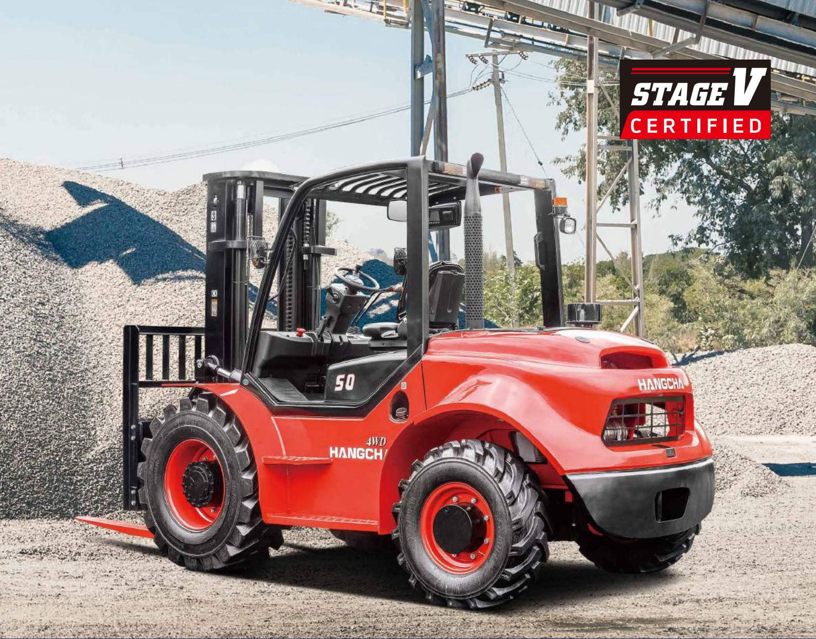
2WD/4WD Rough Terrain Forklift with capacities of 5,000kg
