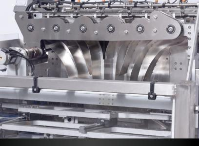
Length: 150" Width: 73" Height: 55" (includes outfeed conveyor) Rate: 50 bags per minute Product size: up to 5" diameter for 6 lanes Electrical: 220V – 15A – 3PH Pneumatic: 10CFM @ 90PSI
