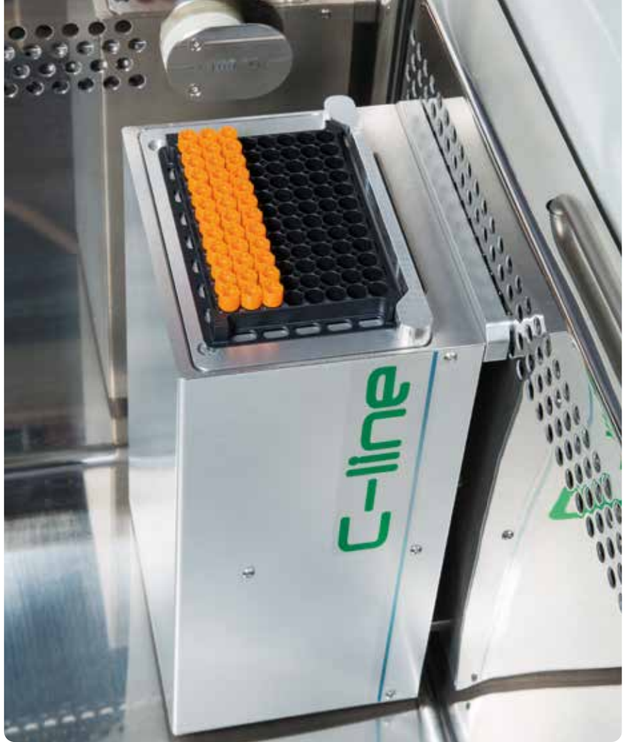
ColdEye installed inside ASKION C-line® work bench to identify samples below –100°C
