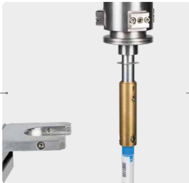
Pick-and-Place-robot above a tray at an ambient temperature below -100^{\circ}\text{C} (left), gripper changing system of HS200 M/L with single gripped sample (middle) and SBS rack gripper (right)
