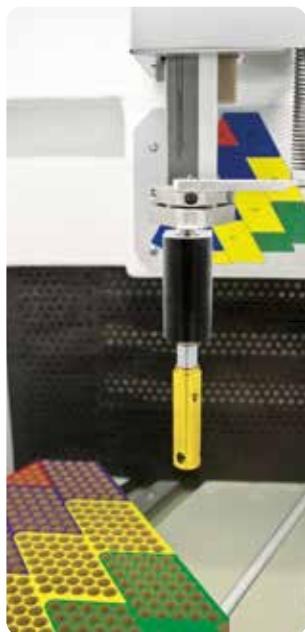
Pick-and-Place-robot above a tray at an ambient temperature below -100^{\circ}\text{C} (left), gripper changing system of HS200 M/L with single gripped sample (middle) and SBS rack gripper (right)
