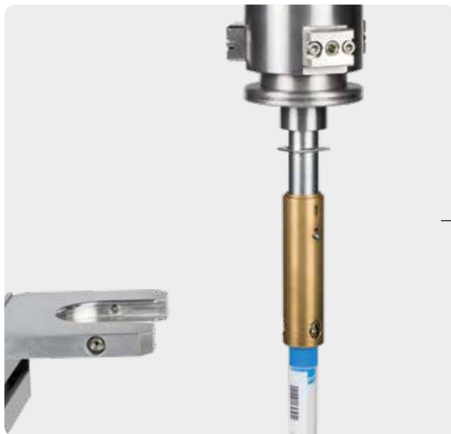
Cherry Picking gripper with a single gripped sample (left) and SBS rack gripper (right)
