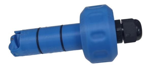
The simple and reliable paddle wheel flow sensor type PWFM is designed for use with every type of solid free water like liquid. The sensor can measure flow from 0.15m/s producing a Highly Repeatable Square Wave output signal. A rugged construction with high chemical resistance and guarantees performance with little or no maintenance required. Dedicated square wave output is available for safe connection to any kind of PLC or Batch Controller.
