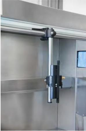
Camera holder mounted to the railing system KA-H-400
