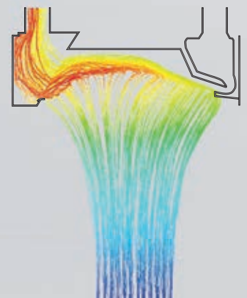
Particle Traces Colored by Particle Residence Time (s)
