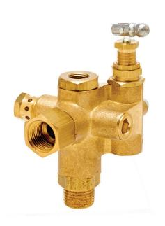
Options include a 1/8" NPT tapped port for throttle control of gas engine, a lockout clip for "dual control" applications, a special 1/8" NPT tapped port for a pressure switch unloader valve, a vent port muffler, and a toggle unloading lever for one-hand warm up control.
