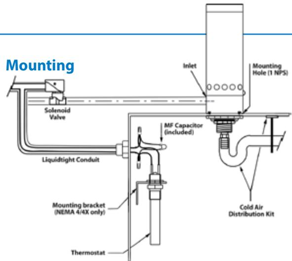
The Cabinet Cooler mounts to the enclosure through a drilled hole or electrical knockout. The NEMA 12 (IP54) Cabinet Coolers may be mounted on the top or side of the panel. NEMA 4 and 4X (IP66) Cabinet Coolers must be mounted on the top of the panel or on the side of the panel using one of our Side Mount Kits (See page 225).
