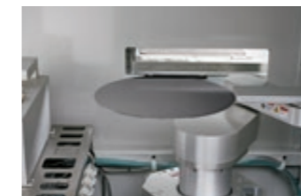
Handling robot loads measuring device with wafers
