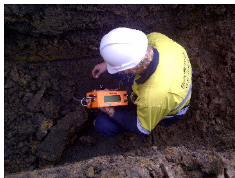
Fig.11 listening to the pipe directly
