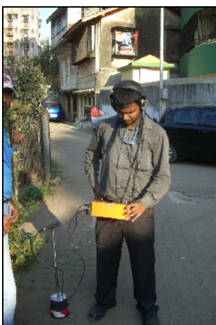
Fig.21 sounding using the Geophone on paving
