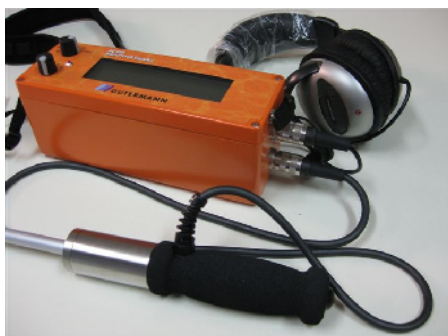
Fig.7 Hand probe connected to Aquascope 550 using the lower binder connector
