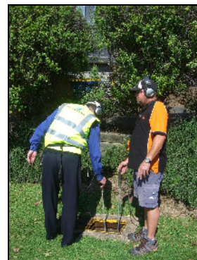
Fig.9 listening directly on a Valve or Hydrant
