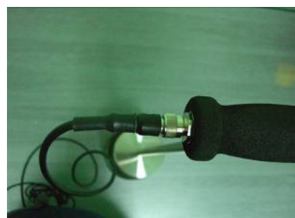
Fig.18 Screw the 4 way plug of the connection cable into the handle
