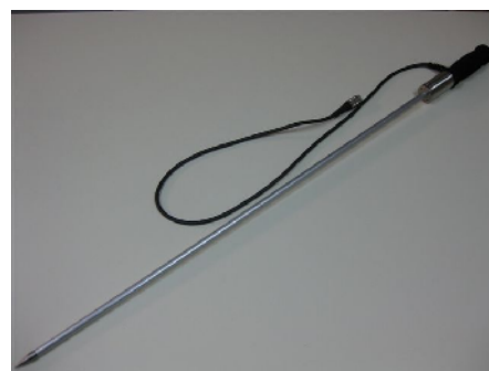
Fig.6 Hand probe Assembly using 2 x rod sections
