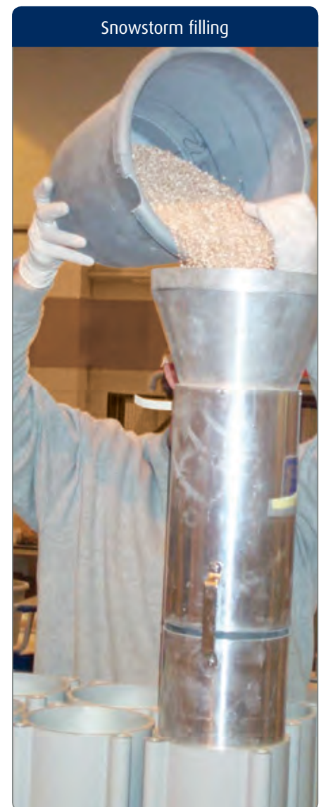
The 'Snowstorm' filling technique ensures consistent dewpoint performance
