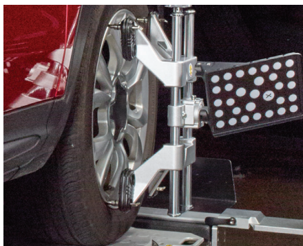
Cast aluminum AC700 wheel clamps fit rims from 11" to 22", with no limitations and 4,9 to 5,2 kg (10.9 to 11.5 lbs.) per clamp.
