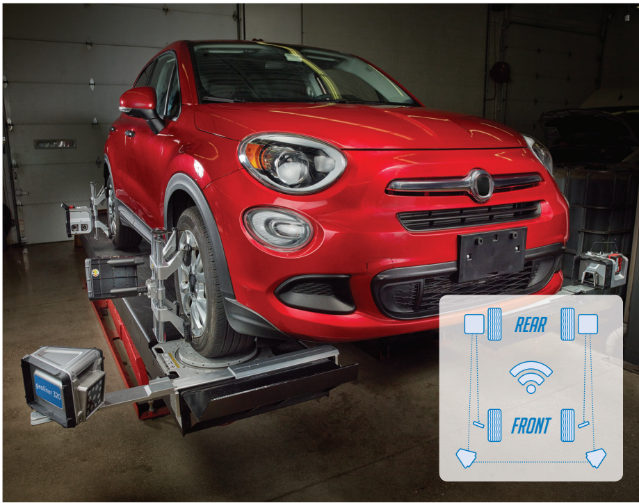
Mounting hardware adapts to common alignment lifts and is easily removed with Quick Release System.
