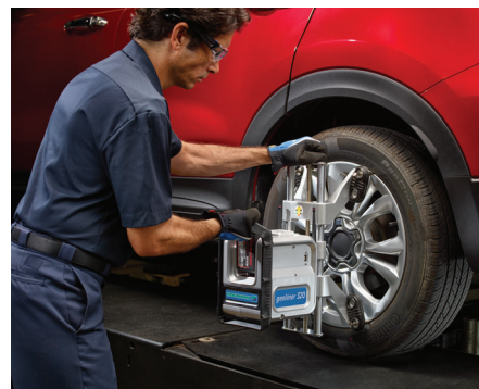
Pods mount with ease, communicating wirelessly and store quickly and easily when finished.
