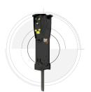
Protect your hammer from overworking. Auto hammer stop warns you after 15 seconds of continuous firing and then automatically shuts it off after 30 seconds – all to prevent wear and tear on the attachment and excavator.
