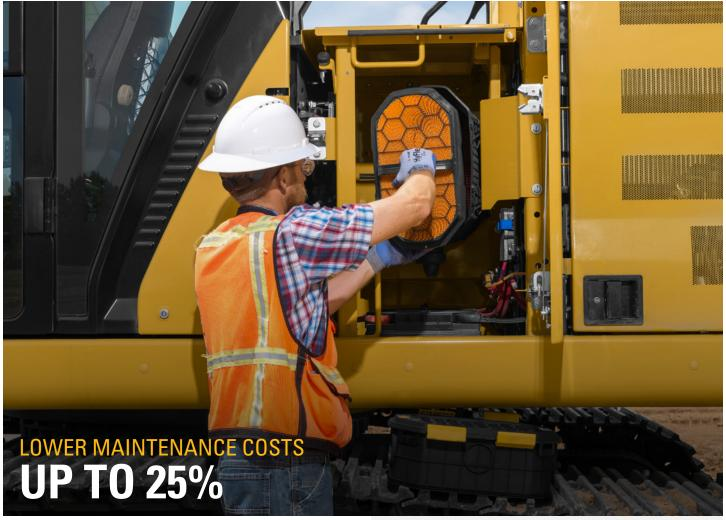
With synchronized and extended maintenance intervals, you get more done at a lower cost compared to the 330F. Consolidated filter locations make service faster. Hydraulic, air, and fuel tank filters have increased capacity and longer life. Access to the operation and maintenance manual is easy through the in-cab monitor.
