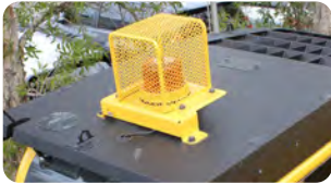
Rotating amber beacon Fitted with factory guard.
