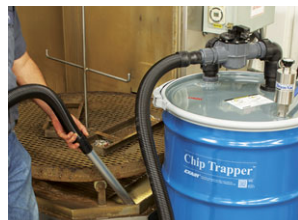
Chip Trapper filters out solids from parts washers.
