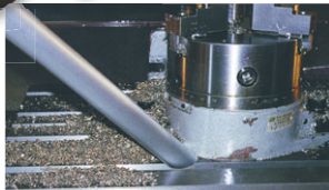
The Chip Vac removes abrasive stainless steel chips from a CNC.
