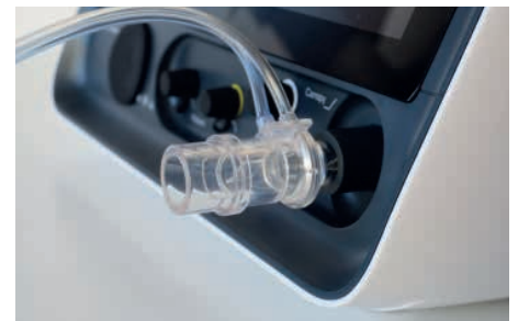
COSMED single-use pneumotach flowmeter (Flow-REE)
