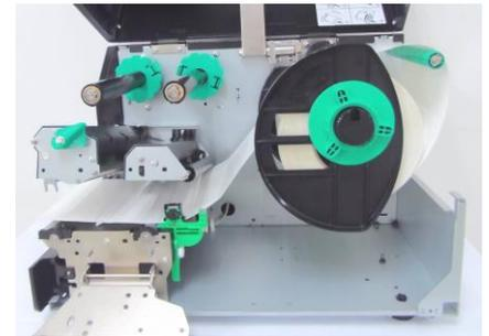
8. Place the media between the Media Guides and adjust them to the media width. Once in the correct position tighten the Locking Screw.
