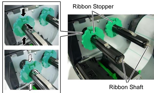
2. Leaving plenty of slack between the ribbon spools, place the ribbon onto the Ribbon Shafts as shown below.
