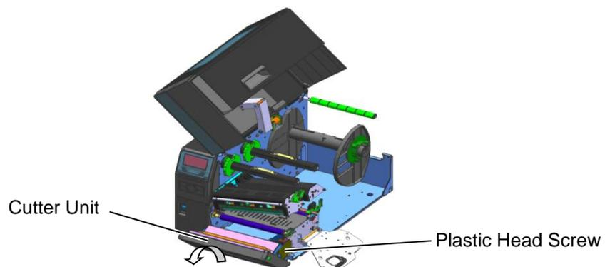
5. Clean the Cutter with a soft cloth slightly moistened with alcohol.
