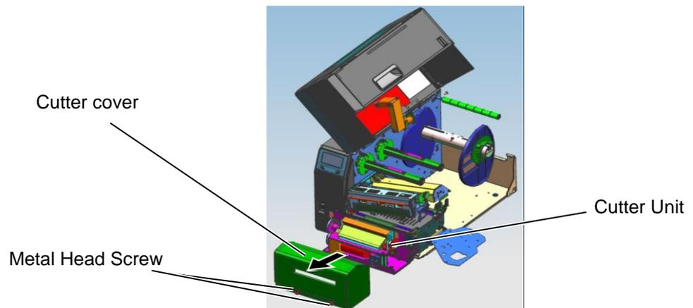
5. Clean the Cutter with a soft cloth slightly moistened with alcohol.
