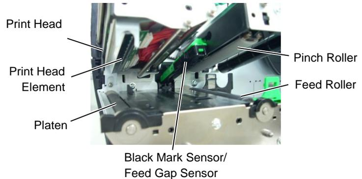
7. Wipe the Platen, Feed Roller, and Pinch Roller with a soft cloth slightly moistened with alcohol. Remove dust or foreign substances from the internal parts of the printer.
