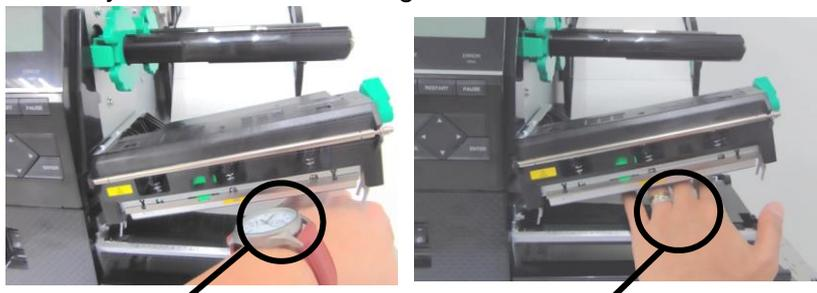
Care must be taken not to allow the metal or glass part of a watch to touch the print head edge.
