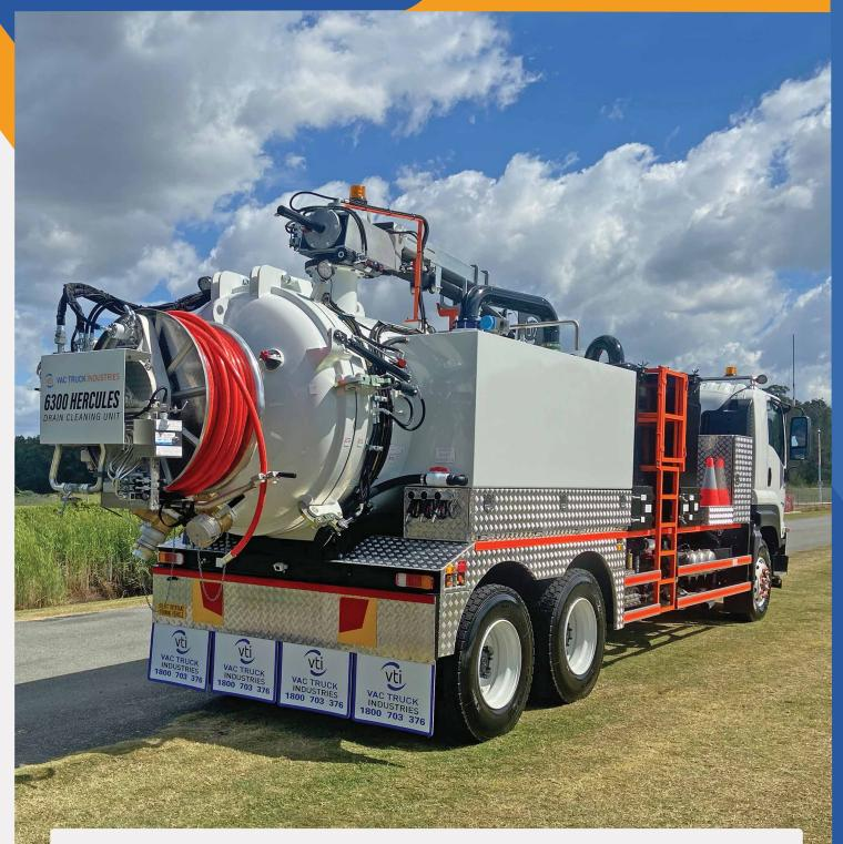
With the addition of the High Pressure DC Jetter Combo system to the already uncompromised power and performance of the HERCULES takes this to next level performance. You can high pressure flush, clear and clean drains and pipes removing from site any collected debris, roots, obstructions and water with high volume vacuum extraction.
