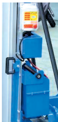
The cable is protected near the motor-housing for safe transportation. Safe lifting point indicated.
