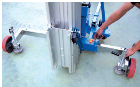
The GL series can be operated on uneven or sloping surfaces. Spirit levels, a variable wheel-base and jacks level and correct setup.
