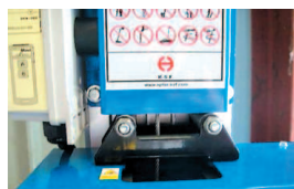
Steel cable is fed through rollers.
