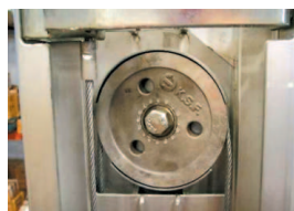
Steel pulleys are used for durability. Pulleys are ringed to ensure operator safety.
