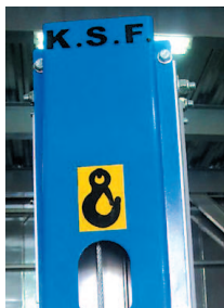
The cable is protected near the motor-housing for safe transportation. Safe lifting point indicated.
