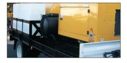
**COMPACT ONE-PIECE SKID DESIGN** The high quality one-piece skid can be easily mounted to a wide range of chassis— permanently, or via container-locks for greater versatility.
