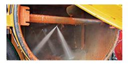
**IN-TANK WASHDOWN SYSTEM.** Saves you cleanup time and makes it easier to remove difficult debris as it delivers a high-pressure water spray to the tank interior while simultaneously dumping material.
