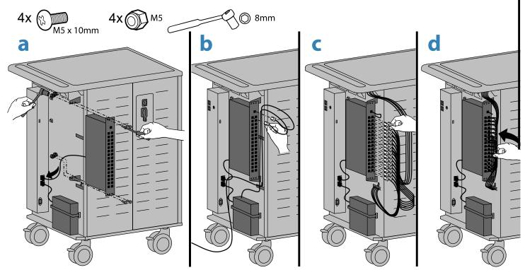
1 O Attach side cover and plug power cable back into cart.
