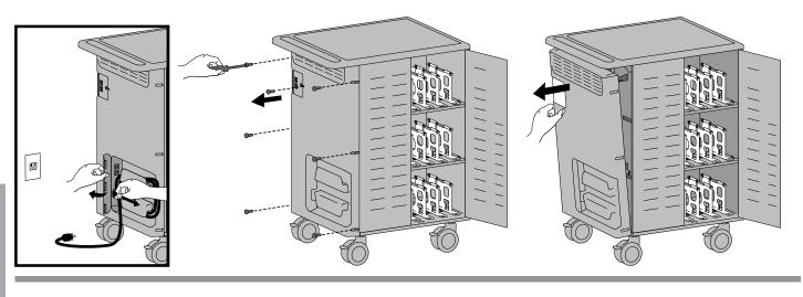
To configure for 30 devices, remove dividers.
