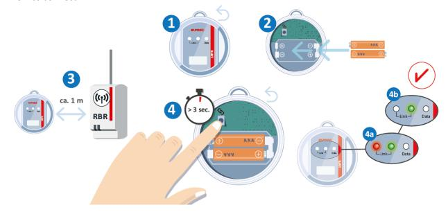
When using the software ELPRO Cloud: Make sure that you have defined the sensor's settings in the monitoring software and that the "Add sensor" wizard shows the image displayed above. This gives you a 10 minutes time frame to connect your module via the following steps:
