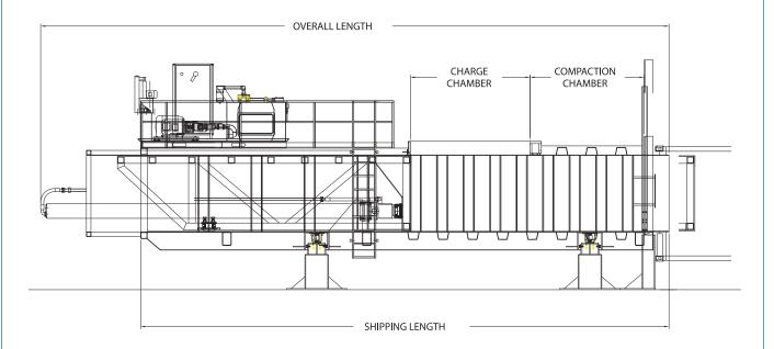
Transfer solid waste more efficiently with a versatile compaction system. SSI's ruggedly constructed compactors consistently deliver the maximum legal payload day in and day out. High density solid waste compaction produces clean, efficient transfer to highway trailers and containers. SSI compaction systems are self-contained units that compact material within the compaction chamber, independent of a transport vehicle.
