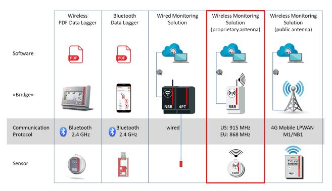
In this factsheet, we mainly discuss wireless monitoring solutions using a proprietary antenna in the 868/915 MHz frequency. This is the most common frequency band available for implementing a proprietary wireless protocol.
