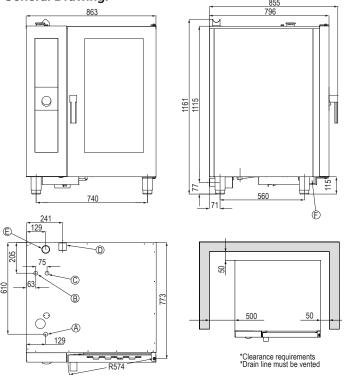
Heat Source: 500mm clearance from an external heat source is required in order to protect the oven control components and allow access to the service panel. For clearances under 500mm, it is mandatory for Stoddart heat shields to be fitted while still maintaining a minimum clearance of 300mm to provide access to the service compartment. Failure to adhere to minimum clearances may void the oven warranty or add service costs due to lack of access.
