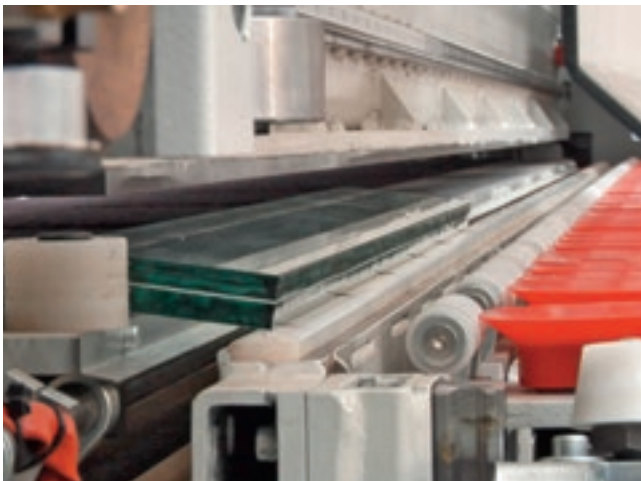
Cutting + breaking + standard removal, 60 mm.
