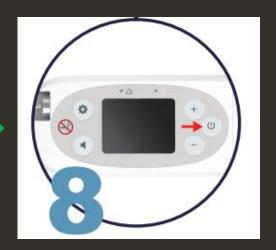
Long press the ON/OFF button for 3 second to shut down the oxygen concentrator
