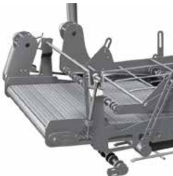
External adjustment of product conveyor and top submerger enable fast turn-around between products, while the M-fryer's low oil volume ensures extended oil life.
