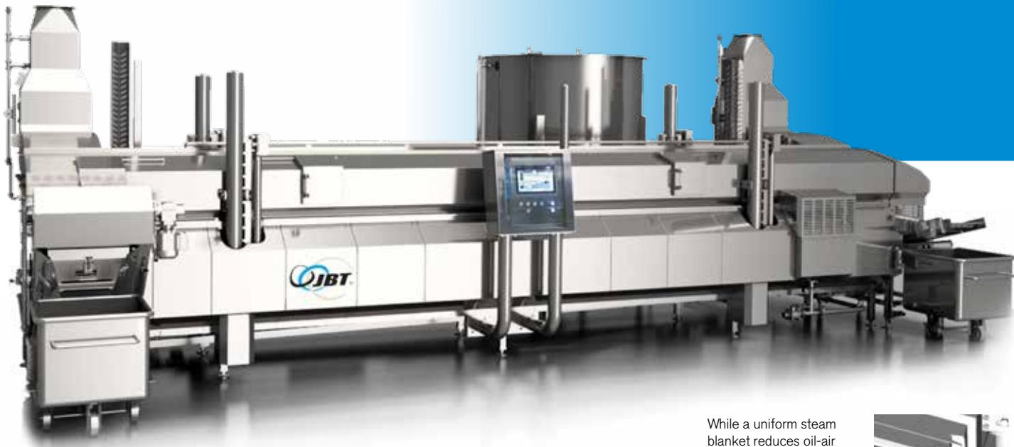
While a uniform steam blanket reduces oil-air contact, the M-fryer's waterlock removes all condensation – better for the oil, better for the food, and better for a safe working environment.
