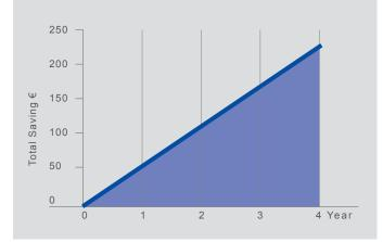
**Example:** ECQ fan with ECQ motor compared to traditional 254 mm fan with shaded pole motor at full time operation and  $\notin 0.15$ /KWh
