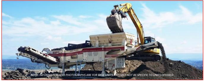
The track mounted M515 trommel is perfect for cleaning dirty material. The unit can handle rocks up to 800mm in size with a capacity of up to 500 tph. It features rapid set up time offering optimal flexibility to move around or to other sites with ease.
