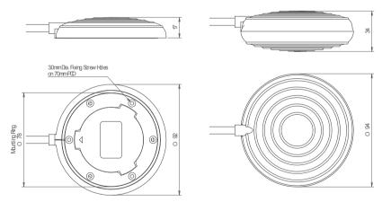
Note: To remove mounting ring from bellows as supplied, insert a 3mm dia. bar in one of the holes & twist anti-cloackwise through 41°. Mounting ring can be used as a template for drilling/tapping holes in mounting face
