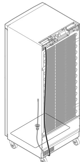
3. Route the cable behind the condenser and push it through the opening until it reaches the desired position.
