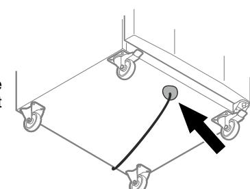
4. Close the sensor cable opening with the sealant provided.
