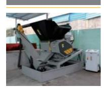
Solid Waste: Cable Wires Usage: Cable Granulator Project: Uniaxial crushing, Conveyor output Area: USA
