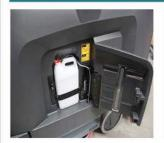
Fitted with a chemical dosing system as standard, this feature saves on excessive use of chemicals.
