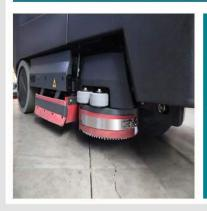
The ASC 260 is fitted with an extendable side brush, used for scrubbing edges and small areas, equipped with guiding wheels for safety in tight spaces.
