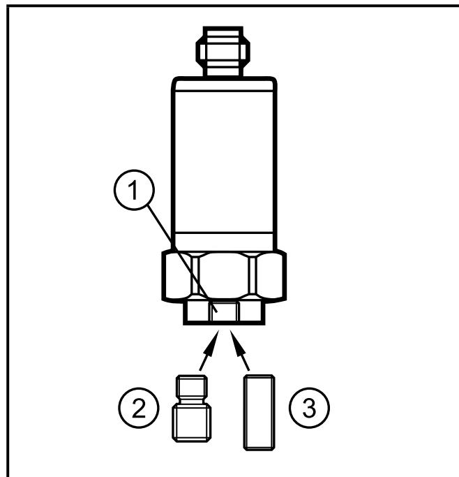
The measuring direction should be in the direction of the main vibration. The main vibration is usually in radial direction to the shaft.
