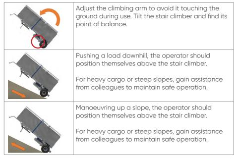
Note: Turn off the power switch when using the stair climber on a slope to avoid inadvertent activation of the climb motor.
